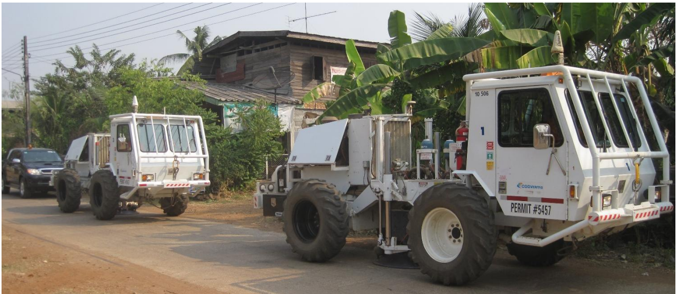
Figure 2 Typical Envirovibe IVI machines to be utilized for EnerCam's seismic program.
