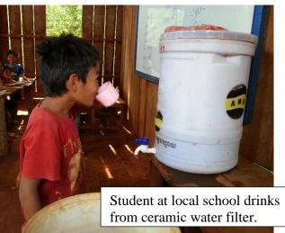
The ceramic filters are made and tested in Cambodia by Resource Development International (RDI), just outside of Phnom Penh, Cambodia's capital city. The filters are portable, effective, and use local materials of clay and rice husk with a coating of silver nitrate on the inside of the ceramic bowl.
