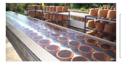
Ceramic inserts of the filter are first kiln fired at 865° C, then submersed in water for several hours before further testing for flow rate, quality control, and application of silver nitrate as a biocide to kill microbes and bacterial.
