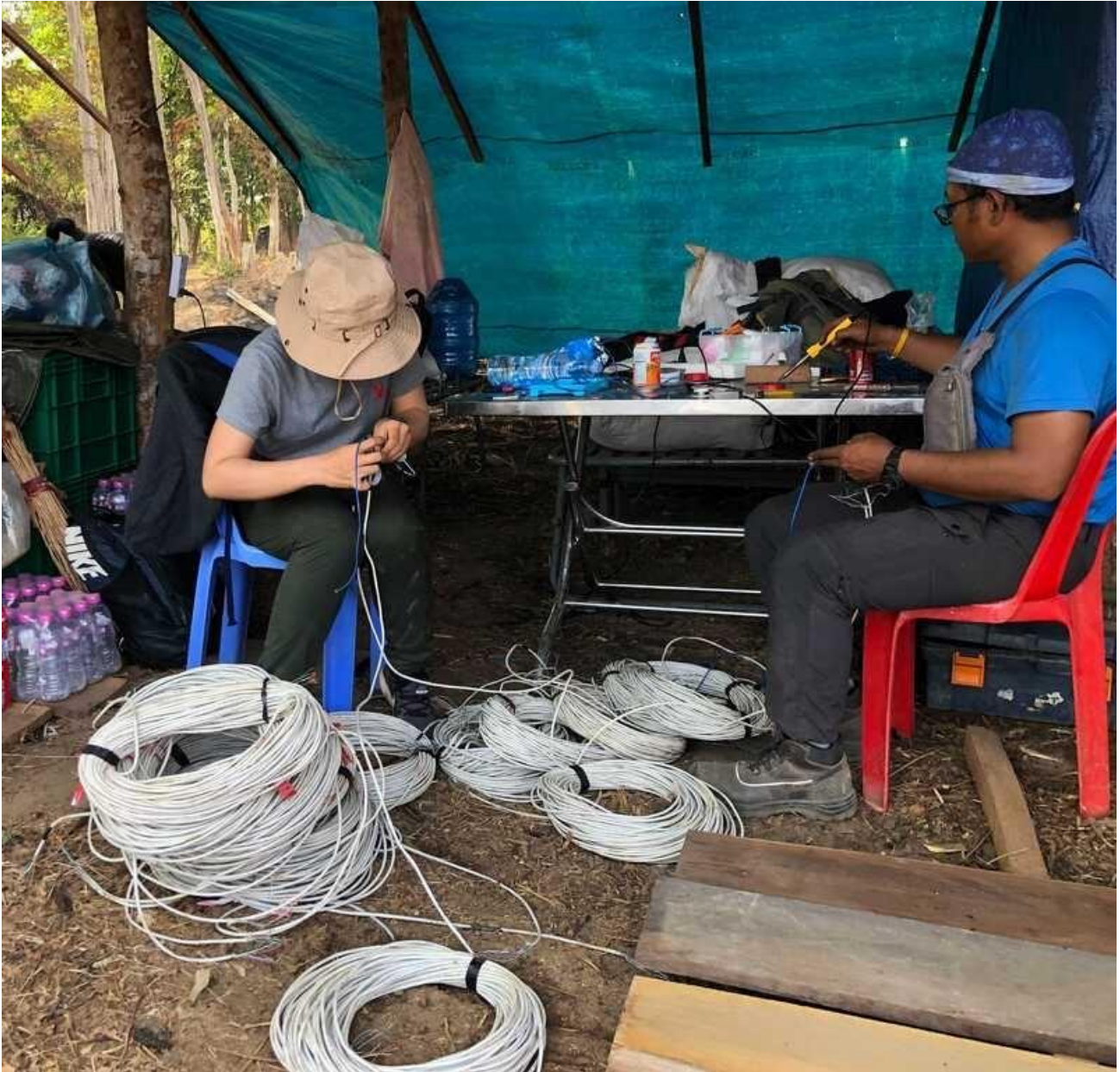
Team members prepare wire for upcoming IP work.
